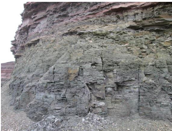
Figure 1. Weathered Keuper Marls in a quarry near Vellberg in Germany.
